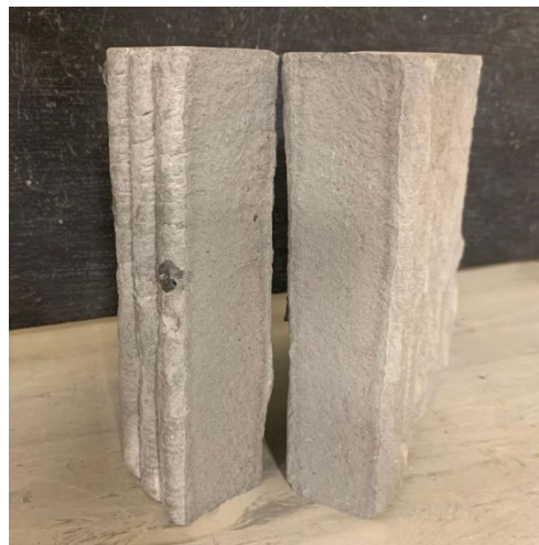
Figure 14. Sample RV1 of vertically restrained test after 4-point bending test
