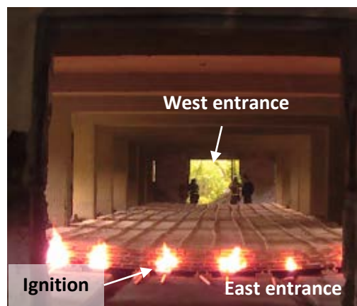
Figure 2. Photos of the final wood crib arrangement used as fuel for the x-TWO experiment. Wood sticks dimensions were 3 cm × 3 cm × 1m. The left image shows a uniform initial linear fire forming and starting to naturally progress. The right image shows completed wood crib at the moment of ignition.
