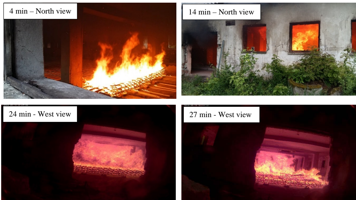
Figure 4. Fire photos taken from different locations (i.e. North entrance and West entrance) at four different times during the Part 1 experiment indicating fire development and progress. An accelerating travelling fire of 32 min duration was observed.
