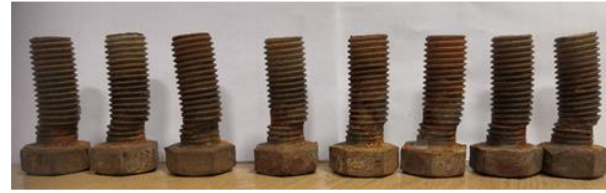
b) Shear deformed lower flange M20 bolts
