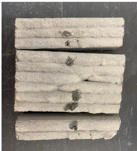
Figure 13. Sample RH2 of horizontally restrained test breaking under hand pressure
