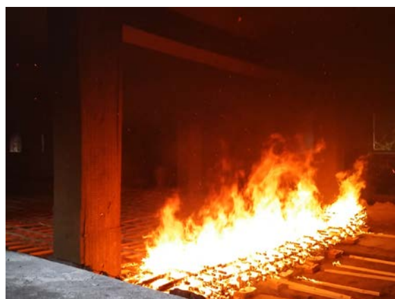
Figure 2. Photos of the final wood crib arrangement used as fuel for the x-TWO experiment. Wood sticks dimensions were 3 cm × 3 cm × 1m. The left image shows a uniform initial linear fire forming and starting to naturally progress. The right image shows completed wood crib at the moment of ignition.
