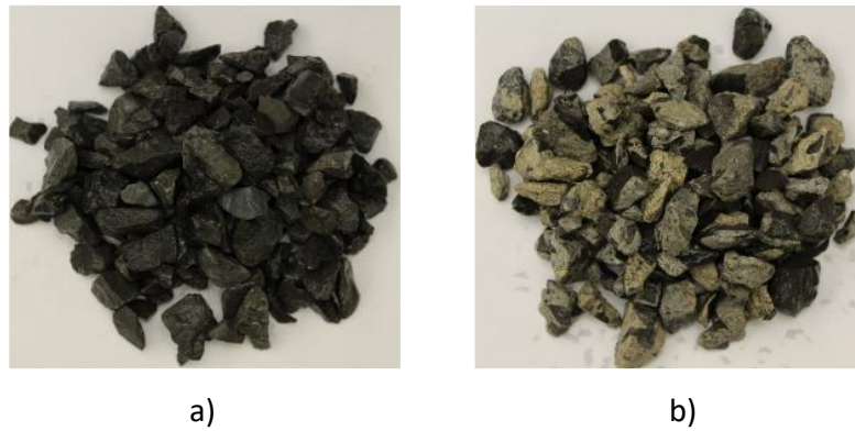
Figure 2. Coarse aggregates types, a) Natural crushed limestone aggregate, b) Recycled concrete aggregate
