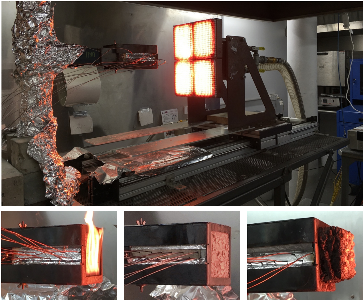
Figure 1. Photograph of the H-TRIS method experimental test setup and of the three types of test samples during testing: (left) unprotected timber, (centre) timber encapsulated with plasterboard, and (right) timber coated with intumescent coating.
