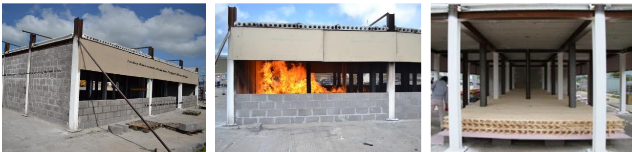
Figure 2. Photographs of the experimental campaign carried out by Ulster University in the frame of TRAFIR project: (a) compartment for test n°2 ; (b) fire at the beginning of test n°2 ; (c) continuous fire load made of wood sticks
