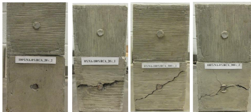
Figure 4: (From left) Pure End-Slip, Block Splitting, Diagonal Splitting, and Radial Splitting
