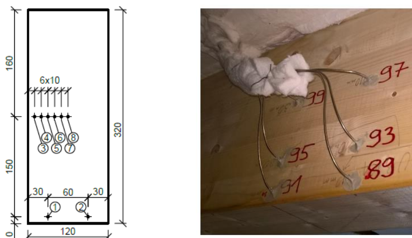
Figure 14. Cross-section of beam 3 and wiring to sensors
