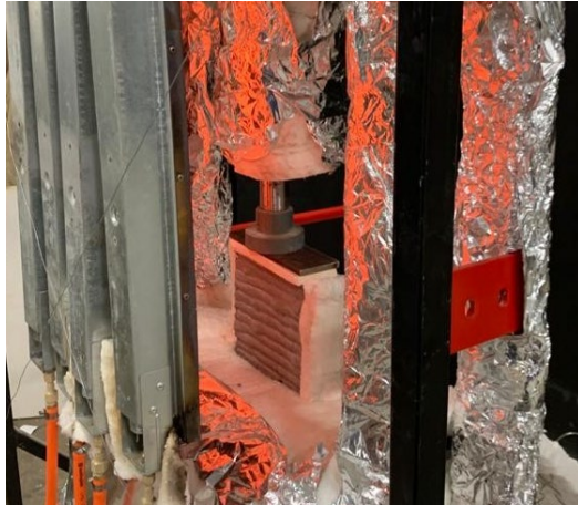
Figure 3. Restrained with layers orientated horizontally (restrained perpendicular to layers - referred to as RH)
