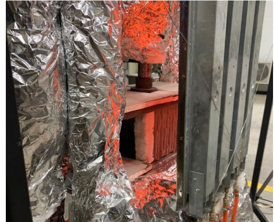
Figure 4. Restrained with layers orientated vertically (restrained parallel to layers - referred to as RV)
