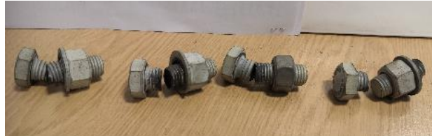
b) Fractured lower flange M16 bolts
