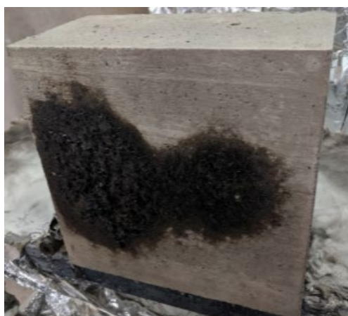
Figure 7. Melted concrete sample.
