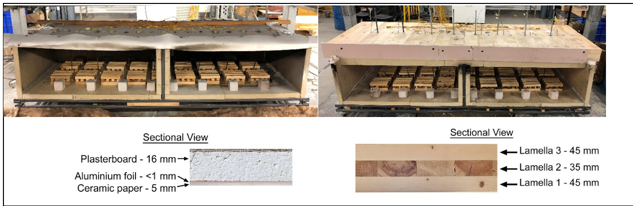
Figure 2 – Compartment with varied ceiling lining: non-combustible (left) and combustible (right).
