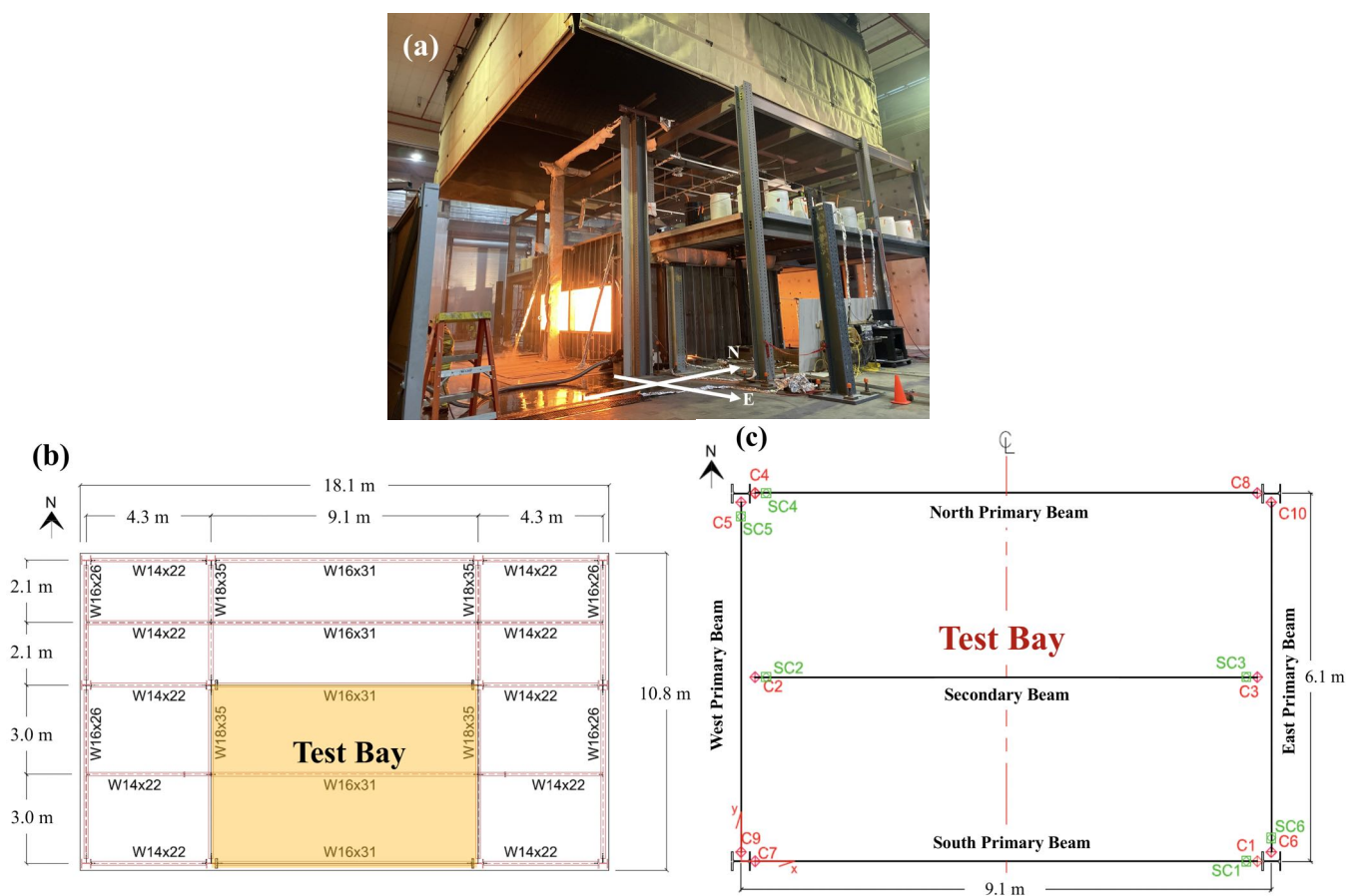
Figure 1. NIST large compartment fire experiment [8] on a steel-composite building. (a). Photo taken during the experiment; (b). Plan view of the test building and test bay location; and (c). Plan view of composite connection instrumentation locations in the experimental compartment, ten in total, from connection 1-10 (abbrev. as C1-C10).
