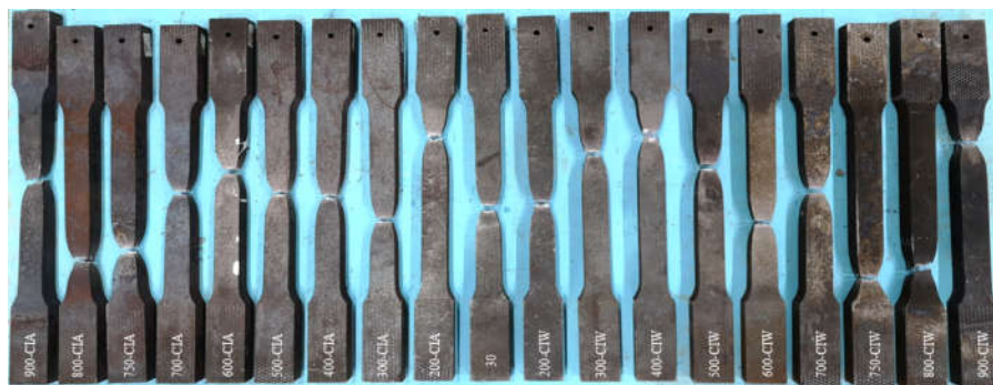
Fig. 3 Superficial color changing of specimens experiencing various heated temperatures
