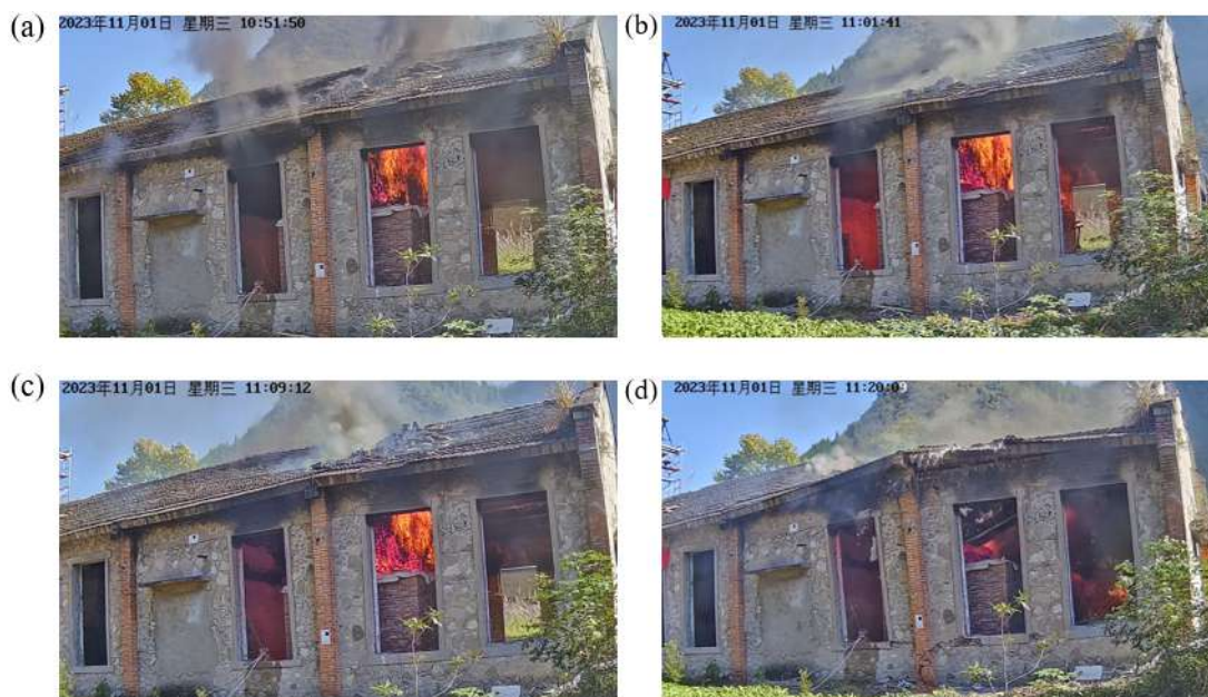
Figure 4 The test process of the fire test (Southwest perspective). (a) 2554 s. (b) 3145 s. (c) 3596 s (d) 4253 s
