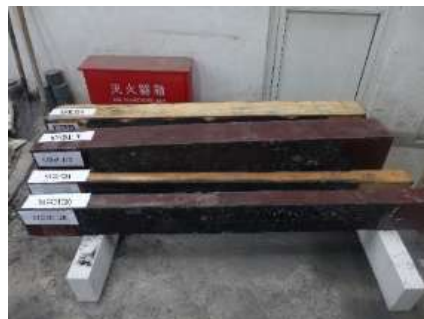
(b) timber beams after 40 mins' fire
