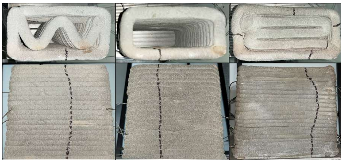
(b) Vertical cracks in the specimens
