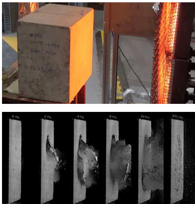
Figure 1. Time-history of incident radiant using H-TRIS for heating conditions tested and example of outcomes of high-speed camera showing the moment of spalling
