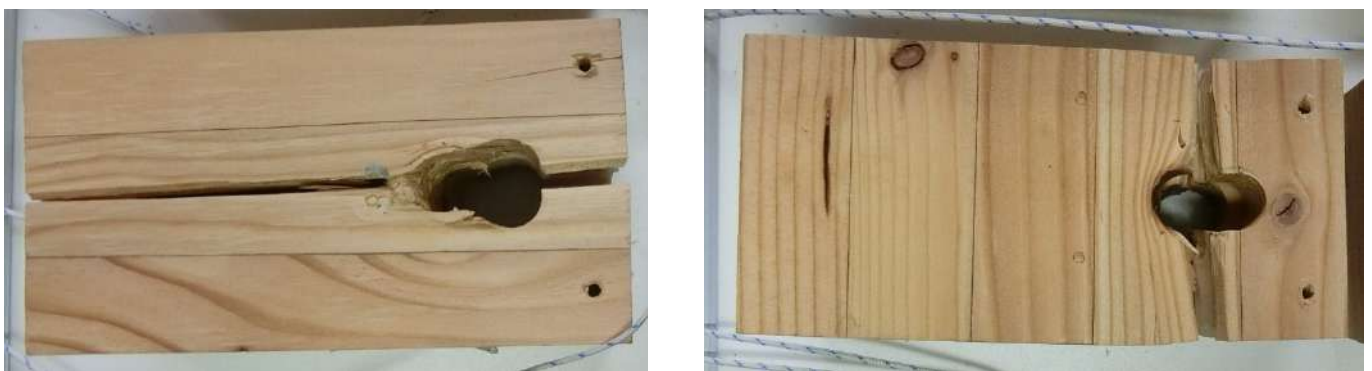
Figure 19. Specimen after the test (TR tests, load ratio 2/3)
