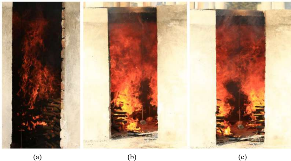
Figure 8: Flashover of SD fire test
