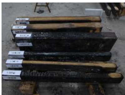
(a) timber beams after 20 mins' fire
