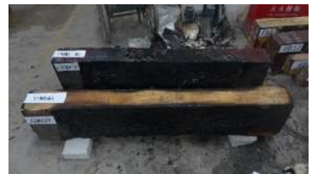
(c) timber beams after 60 mins' fire
