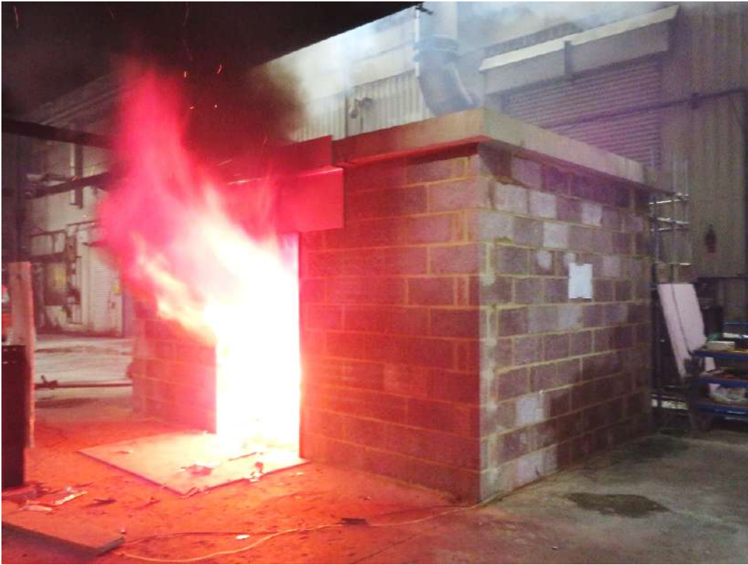
Figure 6. External flaming shortly after flashover
