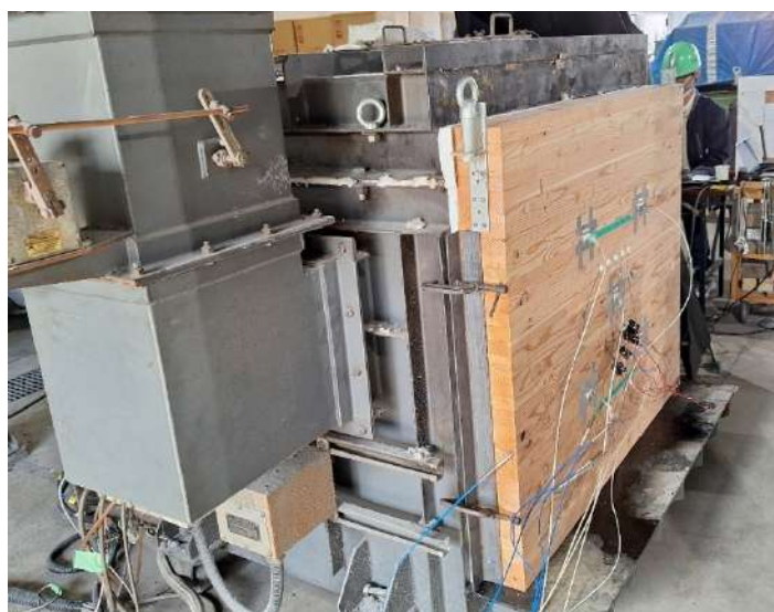
Figure 1. View of the ISO 834 standard fire test using a small box furnace
