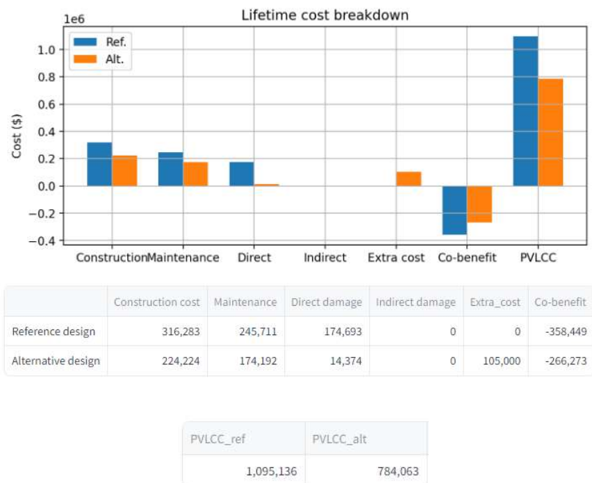
Figure 9 Sample of the outputs of the life-cycle cost estimation for a composite building designed either with a prescriptive (Ref.) or a performance-based approach (Alt.)
