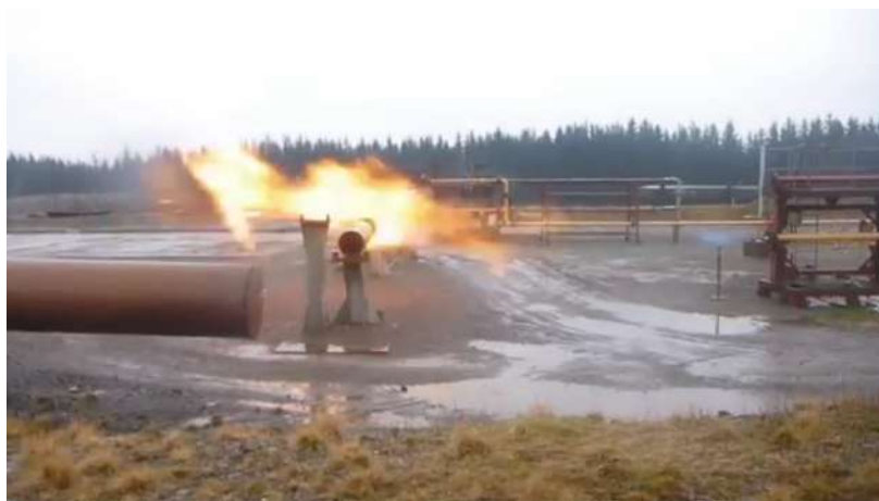
Figure 5. Full-scale jet fire test
