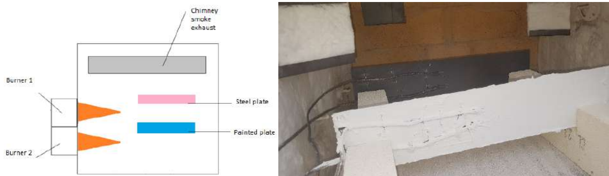
Figure 5. Arrangement of the plates in the furnace for the first test
