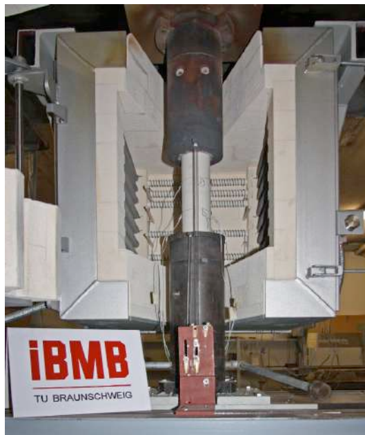
Figure 1. Experimental setup for steady-state and transient-creep tests
