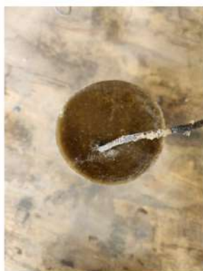
(a) Casted cylindrical specimen instrumented with Type K- thermocouple
