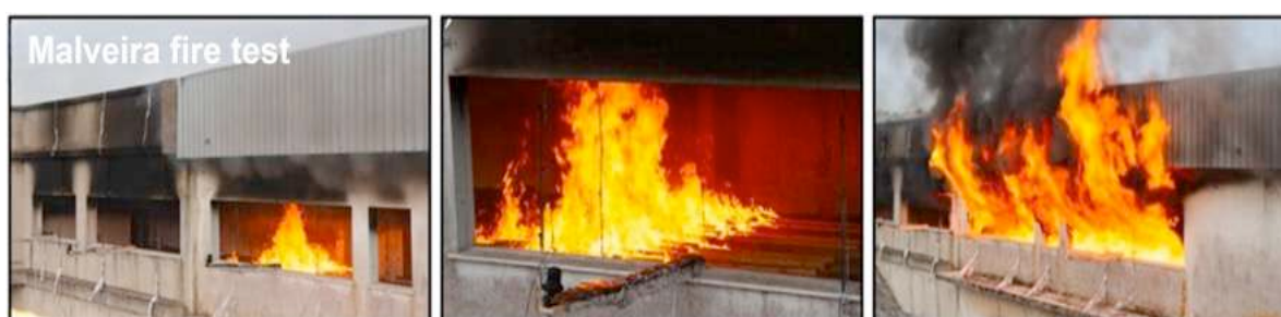
Figure 1. Travelling fire exhibited in Malveira fire tests with non-combustible ceiling [11]
