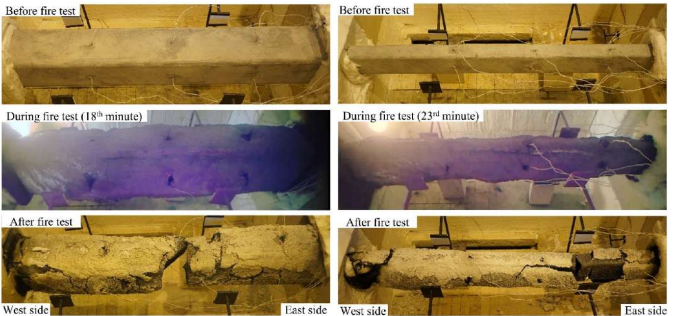
Figure 4. Mechanically loaded specimen before, during and after the fire test; specimen 3C - 220x220x10 mm 3 (left); specimen 4C - 160x80x6.3 mm 3 (right)
