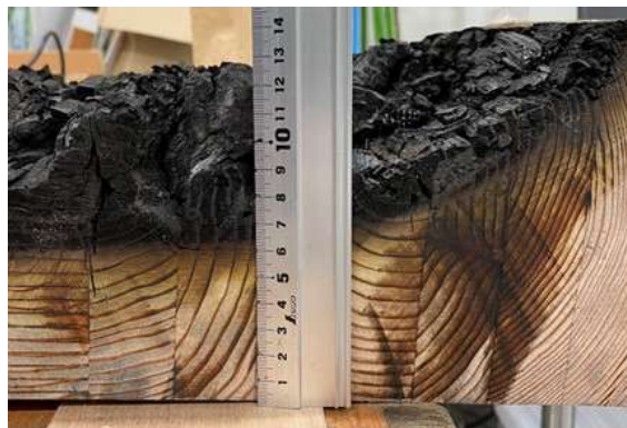
Figure 19 An example of cut section of specimen after test (120+180)
