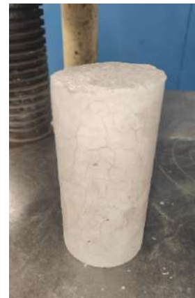
(b) PMC-ATH specimen after heating to 600°C
