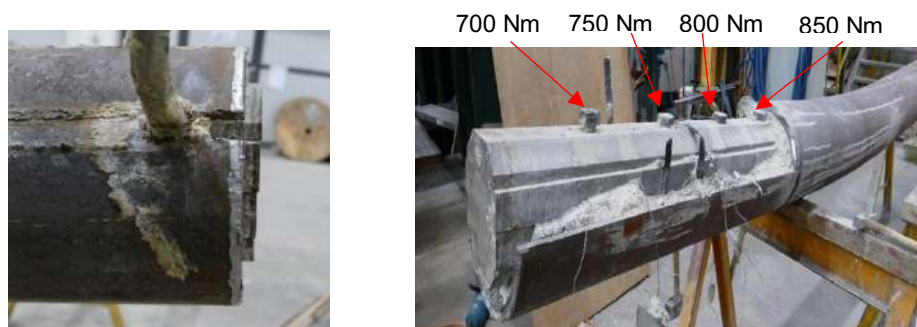
Figure 5. The slip between the sheets of core (left), the torque load used to loose nuts (right)
