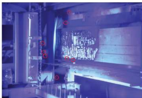
Figure 2. Ember generation of glulam sample tested with a radiant heater (circled) [6]
