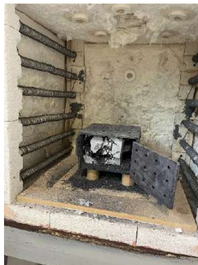
Figure 3. Metallic cage to protect the furnace from explosive spalling
