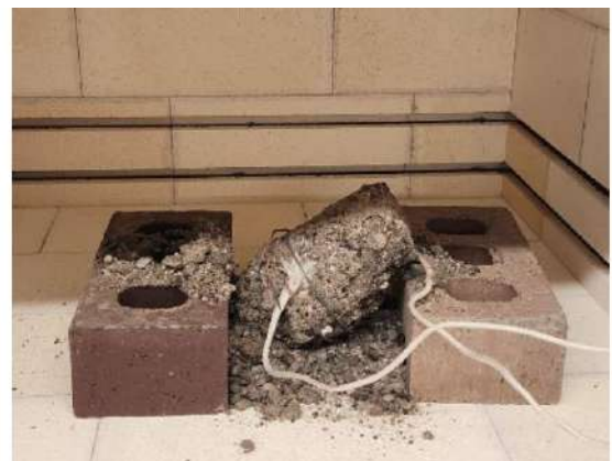
(b) PC-PO-ATH specimen inside the furnace at 400°C
