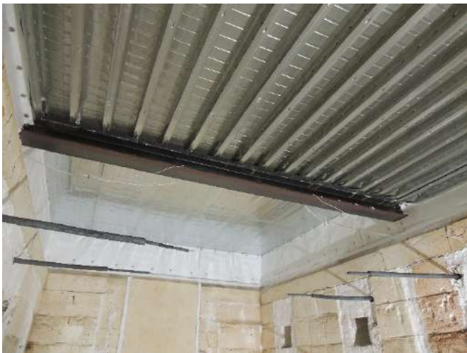
Figure 3. Bottom heated surface of the specimen
