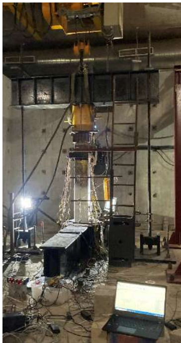
Figure 2. Quasi-static Cyclic Test setup
