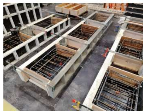
Figure 2. Formwork of the beam-end tests specimen
