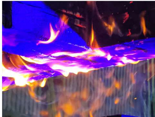
Figure 7. Underside of Connector during fire test
