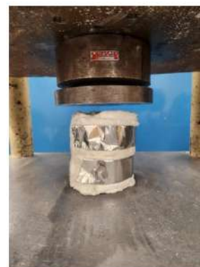
(b) Specimen insulated in a thermal blanket to maintain its hot state while testing
