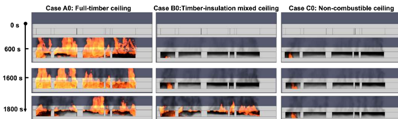
Figure 7. Fire development of the compartments with different ceiling arrangements under continuous fuel load
