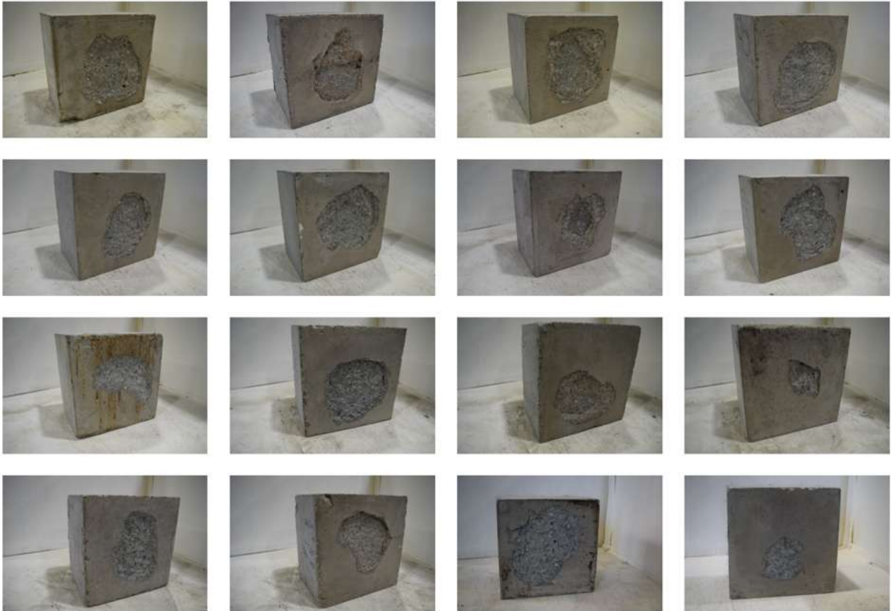
Figure 4. Photograph for each spalled sample after testing
