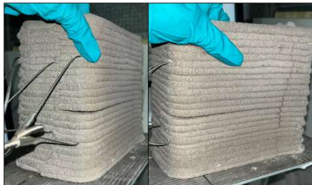
(a) Interlayer cracks in specimen
