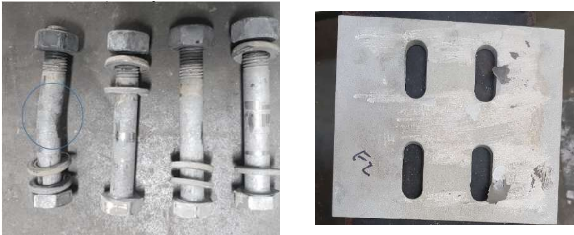
Figure 11. Shear of the bolts (left), wearing of the friction plates (right)
