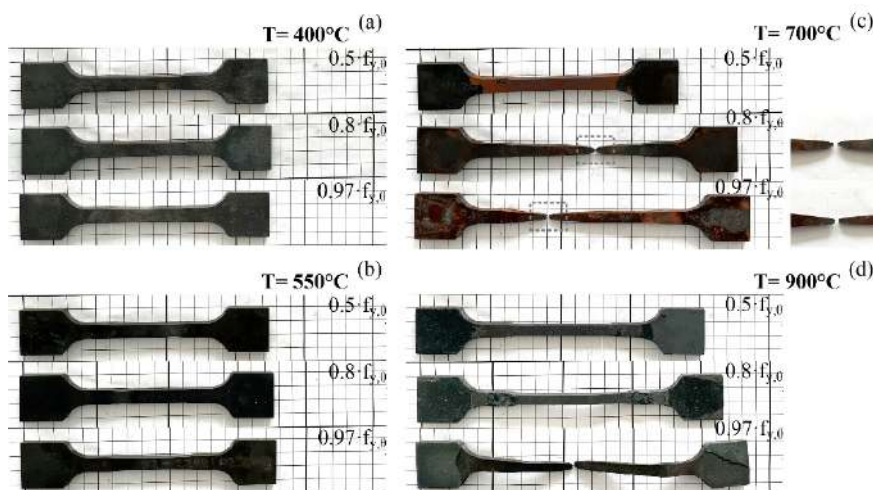
Figure 4. Specimens from creep tests of steel S960QL at a temperature of (a) 400°C, (b) 550°C, (c) 700°C and (d) 900°C
