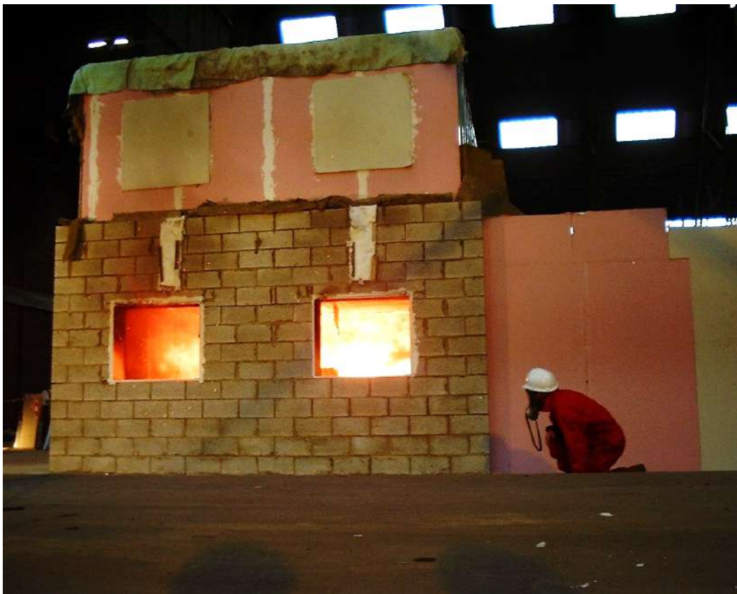
Figure 1. Full-scale fire test of light steel framed house
