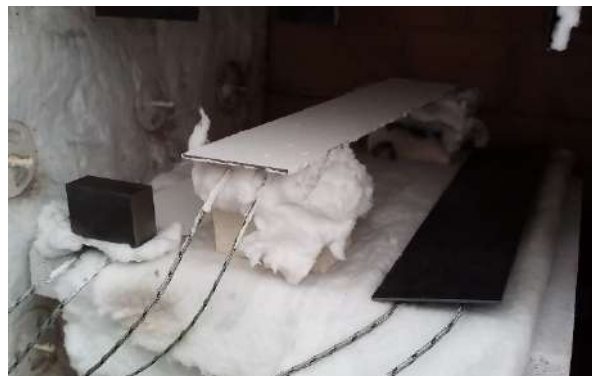
Figure 4. Arrangement of the plates in the furnace for the first test
