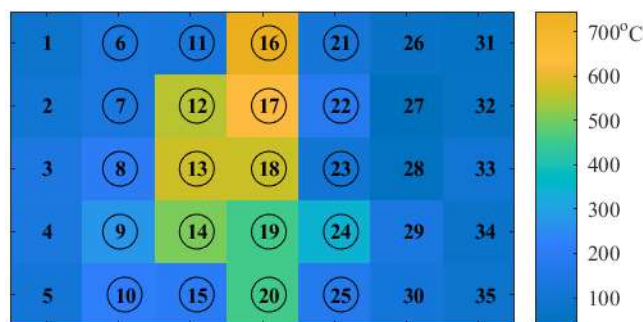
Figure 8. Maximum recorded temperature at different locations over the surface (circles show the locations for post-fire test sampling)
