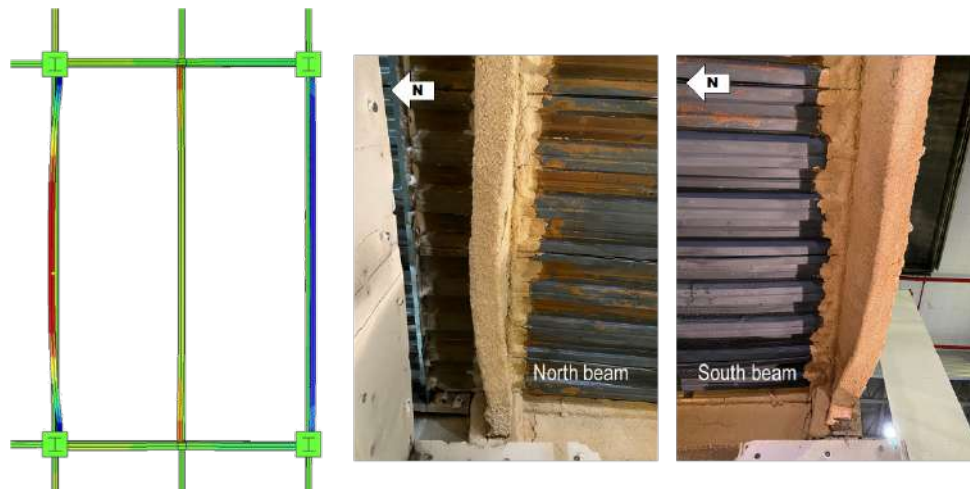
Figure 10. Simulated and observed lateral displacement of bottom flanges of the north, and south W16×31 beams (test pictures are from Choe et al. [4])
