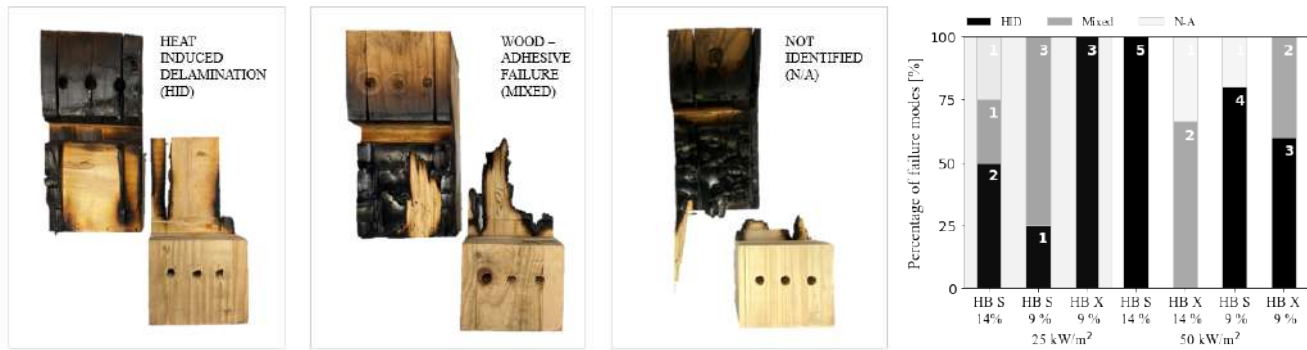
Figure 5. Failure modes (left) and their distribution with the subsets depending on the applied heat flux and moisture content (right)
