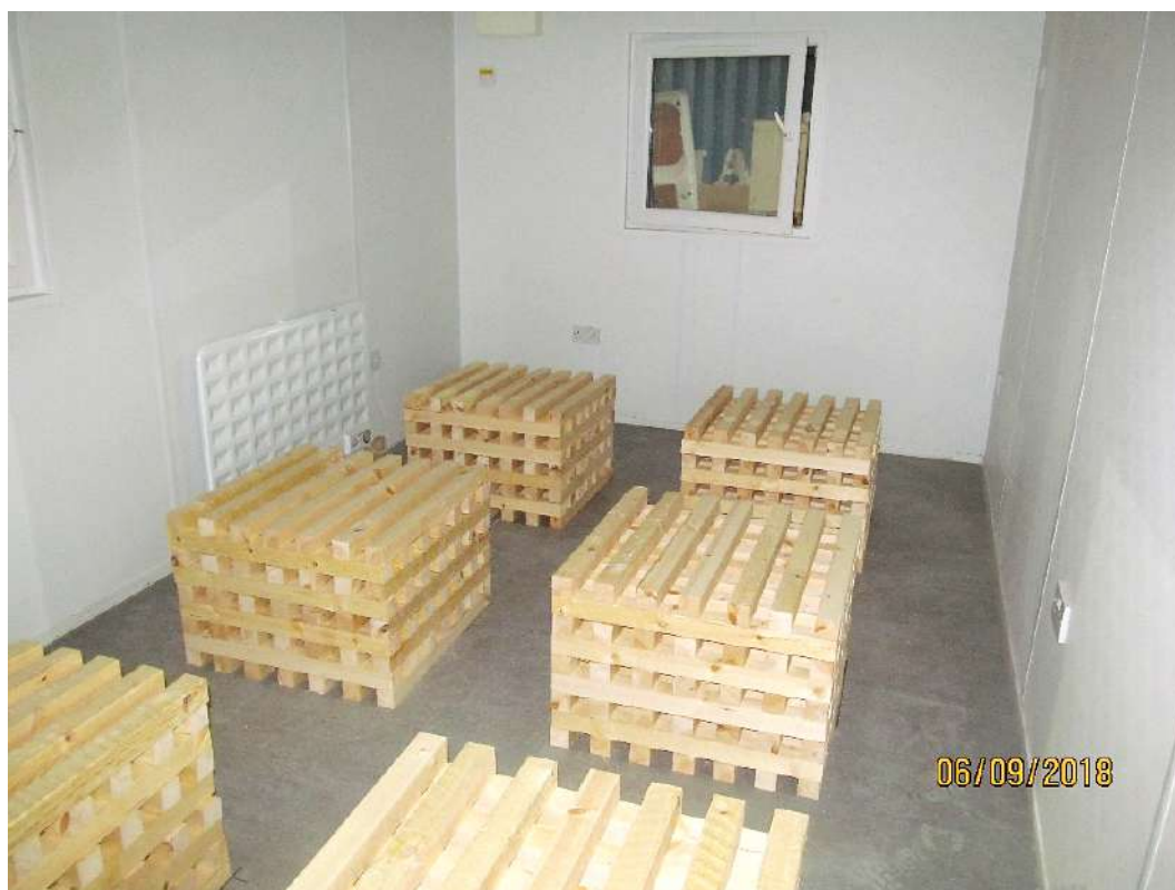
Figure 3. Typical fuel load for a site accommodation unit
