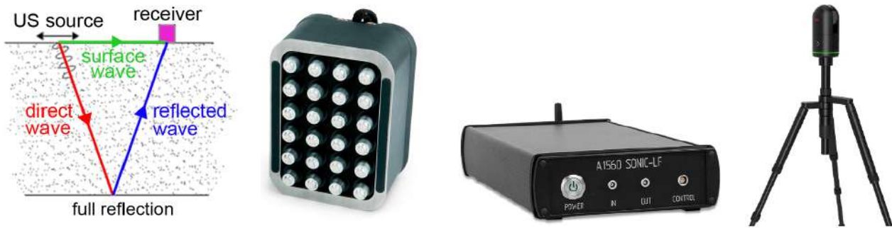
Figure 5. Ultrasonic pulse-echo principle, sensor array (50kHz, shear waves) and wireless pulser/receiver for real-time monitoring of slab thickness and damage; 3D laser scanner for geometrical survey of the specimen after the tests
