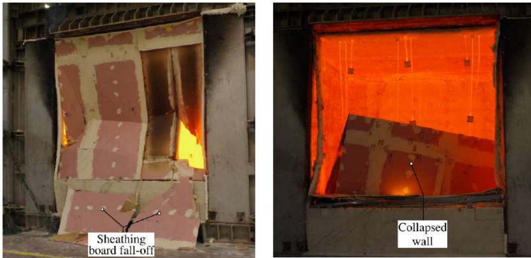
Figure 10. Pictures of LSF wall under testing showing extent of deflection for the one-sided fire exposure condition
