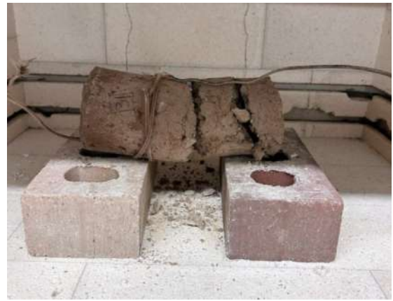
(b) PC-EP-ATH specimen inside the furnace at 200°C
