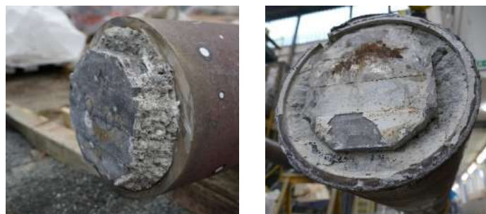
Figure 6. The connection between concrete and core in ambient condition (left), after fire (right)
