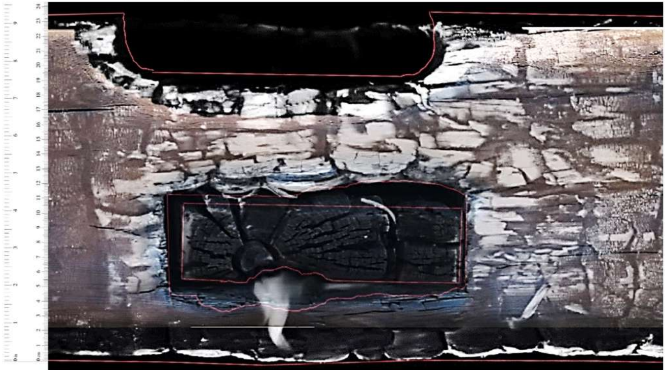
Figure 8. Connector with Original and Damaged States Overlaid
