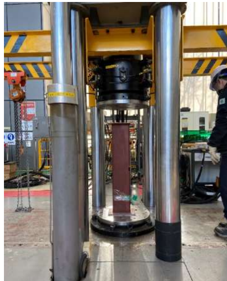
Figure 4. Test set-up of axial loading test
