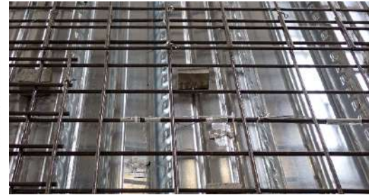
Figure 4. Thermocouples inside the concrete slab
