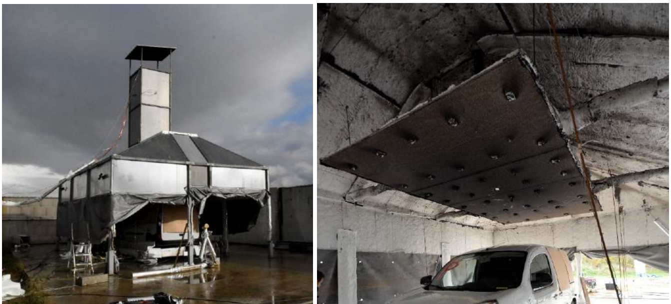
Figure 3. Calorimetric hood (left) and ceiling (right) photos
